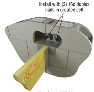
Typical MPH single ply installation
